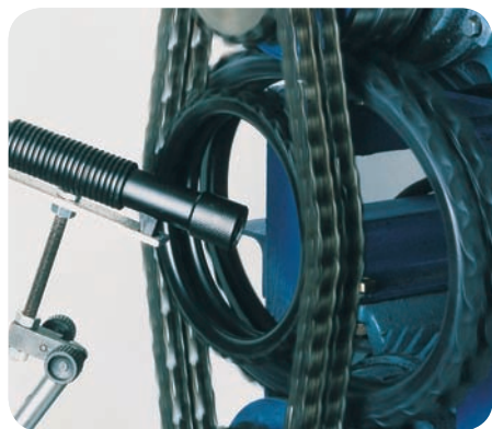
Roll-Ring® kettingspanners in testopstelling
